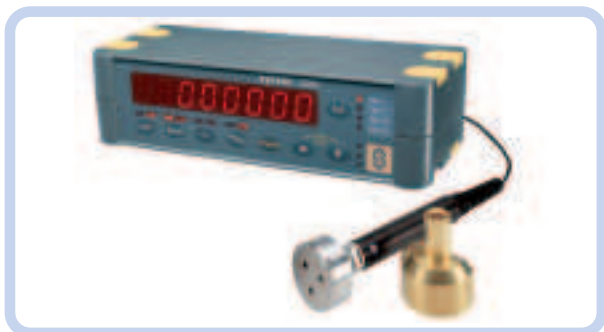
SmartPlug with transducer holder and standalone display
